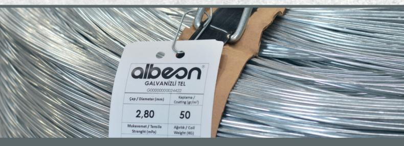
**HOT-DIPPED GALVANIZED STEEL WIRE**
